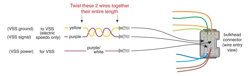
ELECTRIC SPEEDOMETER WIRES: These wires should ONLY be used only if your car has an electric speedometer. Plug them into the main connector as shown here or, on pages 2, 4, or 6 (depending on the proper application for your car) of this instruction set and route them as outlined below.
